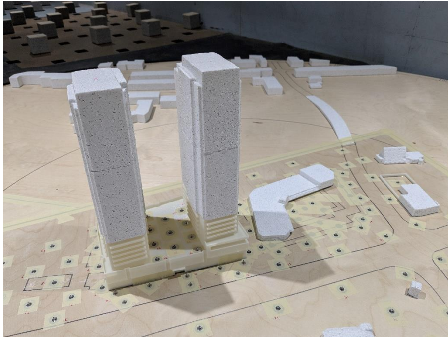
PHOTOGRAPH 5: CLOSE-UP VIEW OF PROPOSED PHASE 1 STUDY MODEL LOOKING SOUTH
