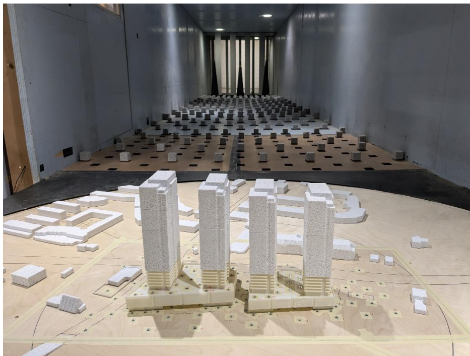
PHOTOGRAPH 4: PROPOSED STUDY MODELS INSIDE THE GWE WIND TUNNEL LOOKING UPWIND
